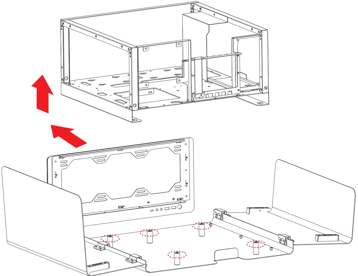
Loosen the five screws, pull the bareness chassis to the front panel direction and take off.
