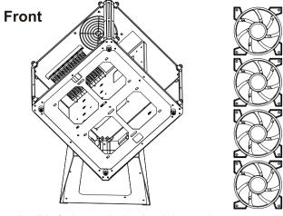
Install the fan between the chassis and glass panel.
