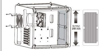
Install the radiator at the chassis inside.
