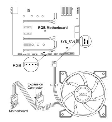
Plug the RGB fans 4pin connector into your motherboard RGB header. You can adjust fan light colors with your compatible RGB motherboard software
