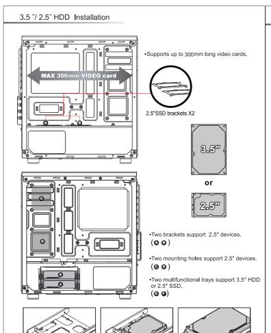
Secure 2.5" SSD / HDD with screws. Secure 3.5" HDD with screws.
